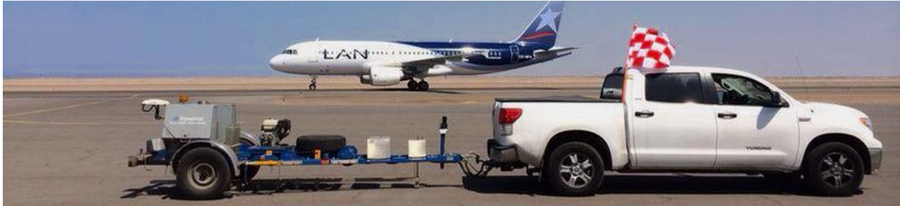
Figure 4-1 Dynatest Heavy Weight Deflectometer
