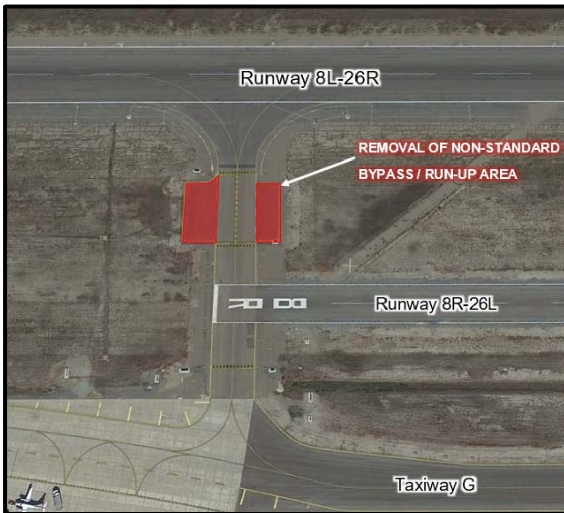
Figure 4. Removal of Non-Standard Bypass / Run-Up Areas
